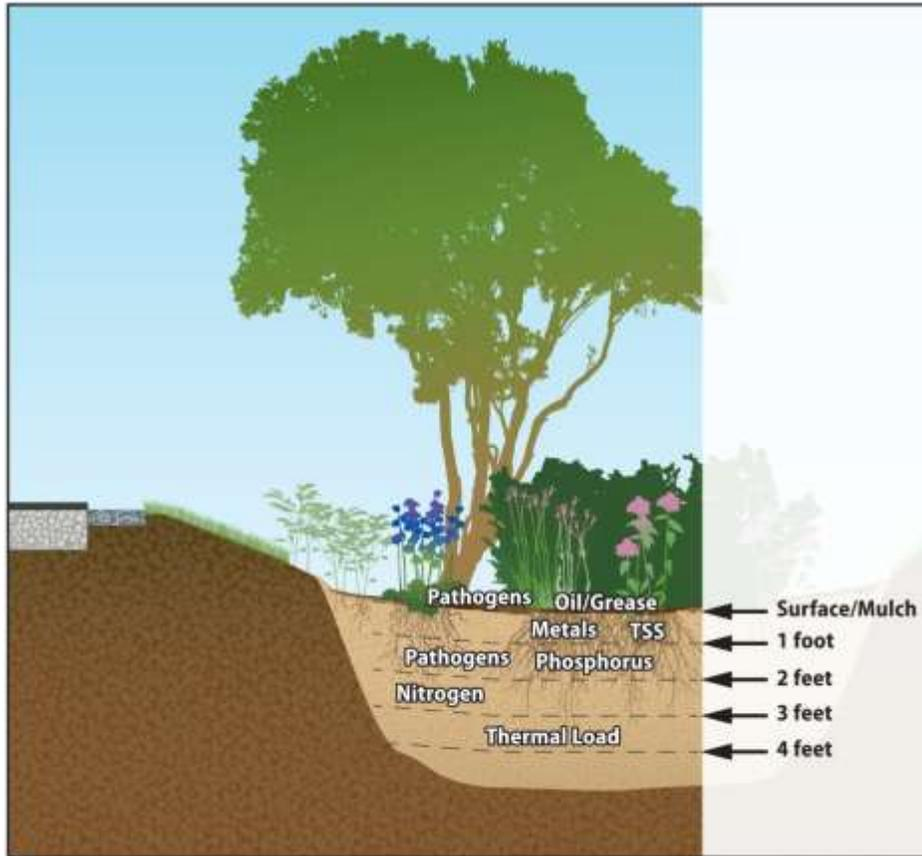
Figure 3-2. Pollutant removal depths in a bioretention area.
